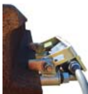
01-086001 Axle Counter swung 120+ deg. away from the rail to allow the 60Kg rail profile to be reground.
