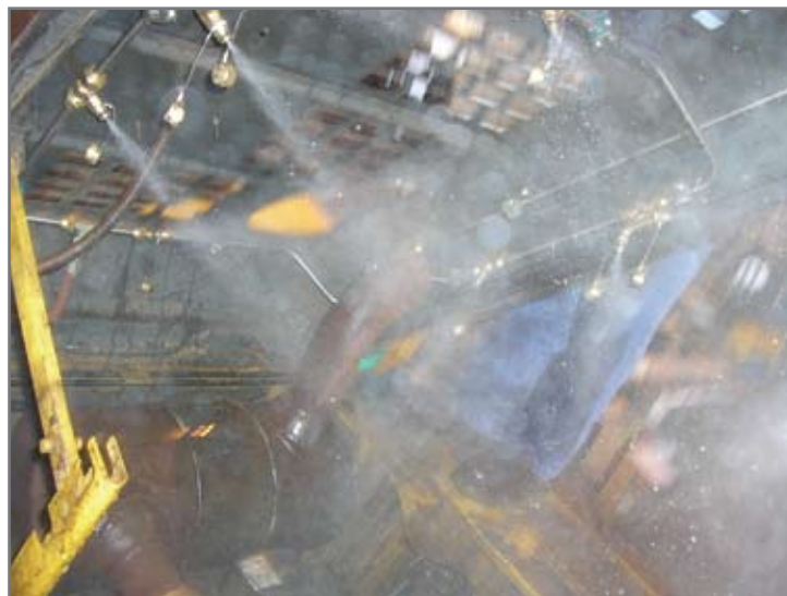
Spraying of foam on engine
